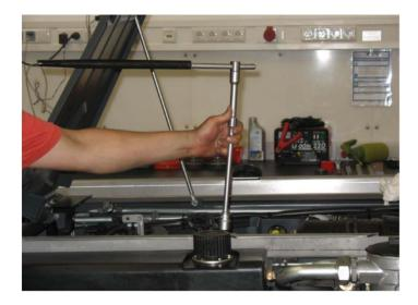
Disassemble the shock absorber - 3 - at the axle.
