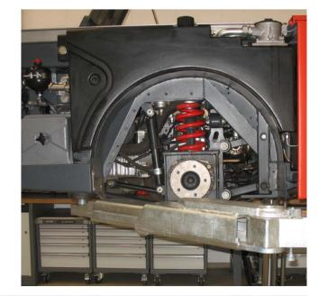
Disassemble the shock absorber at the vehicle frame and axle.
